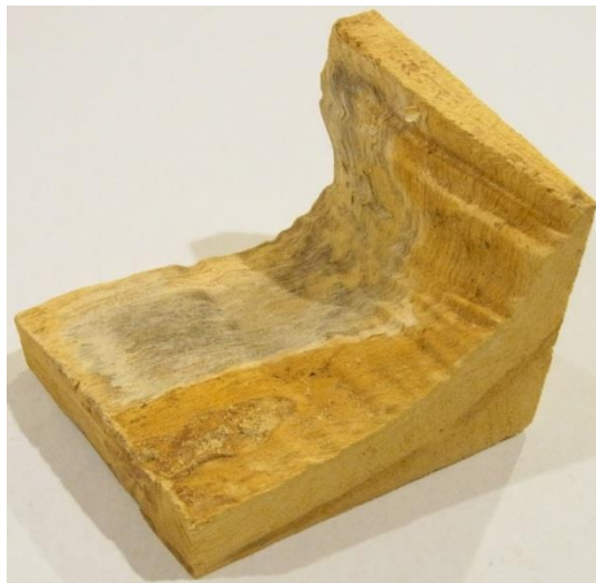
A sample of Crows Ash flindersia australis (Australian Teak) timber. 7.5x6.0x5.8 cm.
