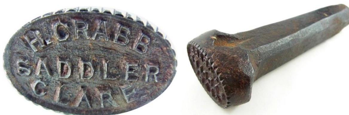
Steel saddle-maker's stamp used in Clare, second half of the 19thC. Length 12.4 cm.
