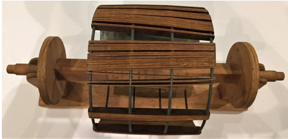
Unbranded smocking machine. 32 cm long, the metal barrel is 12 cm in diameter.
