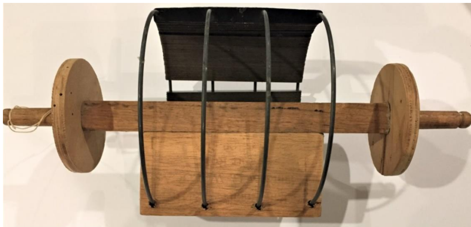
G W Lucas smocking machine. 30 cm long, the metal barrel is 12 cm in diameter.
